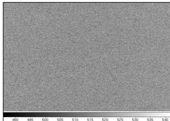
Fig. 3. A bias frame shows a uniform distribution
