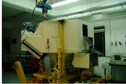
Figure 2.5: ISIS spectrograph off the telescope (© Javier Méndez).
